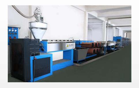
\*This step for producing PE or PP Mono yarn, one machine production per day can provide 3 netting machine material.
