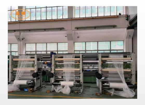
Conditions of film: The film must be smooth and without fold. The thickness of film is 0.05mm  $\sim 0.06$ mm. Blown film is better to the machine.
